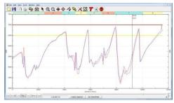
Evaluating RPM data can be used to analyze engine performance. Gearing, shift time, and engine acceleration curves are commonly looked at to improve the racecars performance as well as reduce the potential wear on your equipment.
